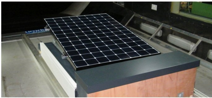
Picture 1: Wind-tunnel test VKI
