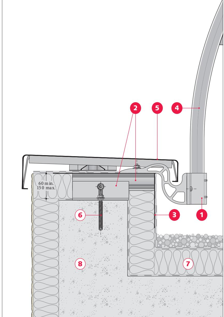
**Fixing to parapet wall using shoe Z**
