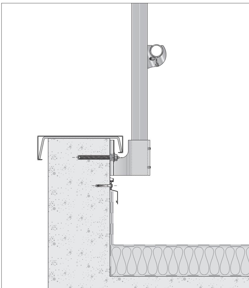
**Fixing to insulated parapet wall with shoe Zc (shoe Z + fixing bracket for insulated parapet wall)**
