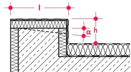
For fixing to roof slab or steel panel roofing: Distance from the inside of the parapet wall to the centre line of the shoe
